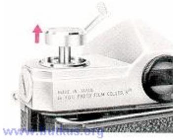
Lift the Combination Film Rewind Crank - Camera Back Lock (14) until the Camera Back (31) opens with a snap. Now take out the cartridge and send it to the processor - the sooner the better
