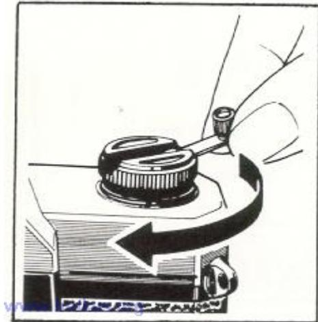
Erect the Film Rewind Crank (14) and wind it in the direction of the arrow to return the exposed film back into the cartridge. Just before the end of the film is reached, you will feel a slight tension release on the crank. Give it two more turns into the cartridge.
